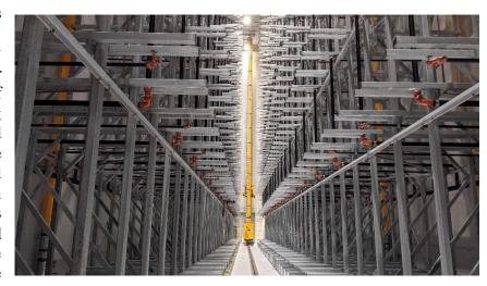
Figure 2: The automated shelving and retrieval system in the vaults of the new Preservation Storage Facility in Gatineau.
